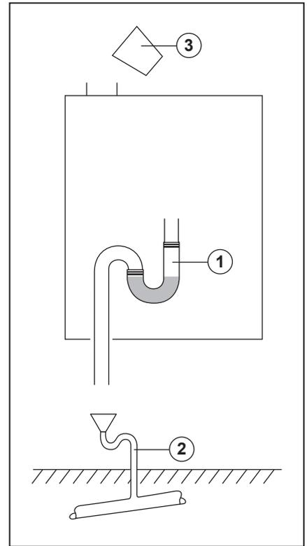
For a cascade system, fit a pipe work header for the condensate drain behind the hydraulic system. For that purpose, the flange plates have holes allowing the installation of a PVC drain of  $\varnothing 40\text{mm}$  max. Use this drain to connect the individual condensate drains of each boiler.
