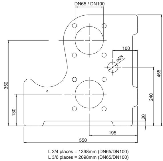
Dimensions low loss header DN100 until 1000kW
