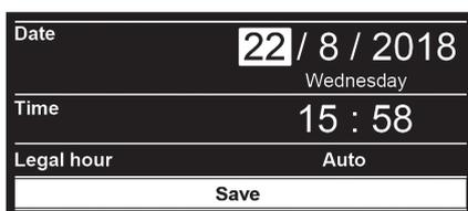
5 Use “+” to go down and “-” to go up to highlight the desired field. Press **OK**. The relevant field starts to flash. Use “+” to go down and “-” to go up to highlight the correct value. Press **OK**. After correctly filled in all fields, Press **Save**.
