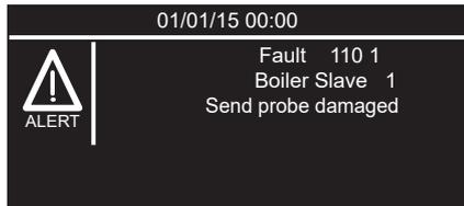
Error from slave boiler 1 indicated on the master boiler.
