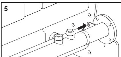
1. Position the pipe work header against the wall. When using several pipe work headers: couple the pipe work headers and supplied gaskets, M12 (DN65) or M16 (DN100) bolts, spring washers and nuts. Align the pipe work header(s) horizontally using the adjustable feet.
