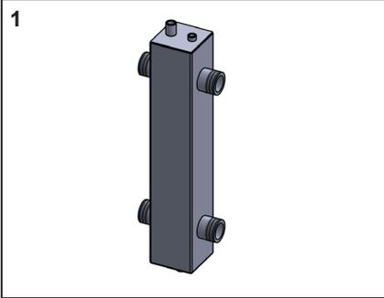
The pipe work headers are available in 2 dimensions, i.e. DN65 and DN100 and are connected to one another by the flange couplings and gaskets, M12 or M16x55 bolts, spring washers and nuts. The low loss header and the complete installation can then be connected to it.
