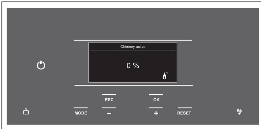
During the combustion check on low load, the speed of the fan should be checked. See the diagnostics procedure on the previous page on how to access the menu during chimney sweep procedure.
